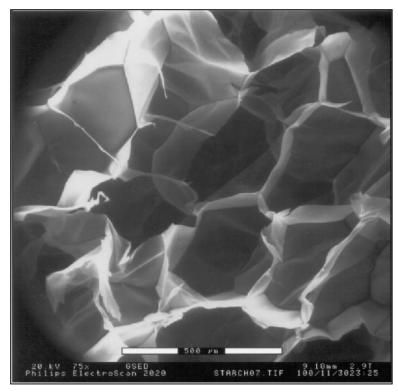
Closed-Cell Structure Cell Size 200 – 500 μm
