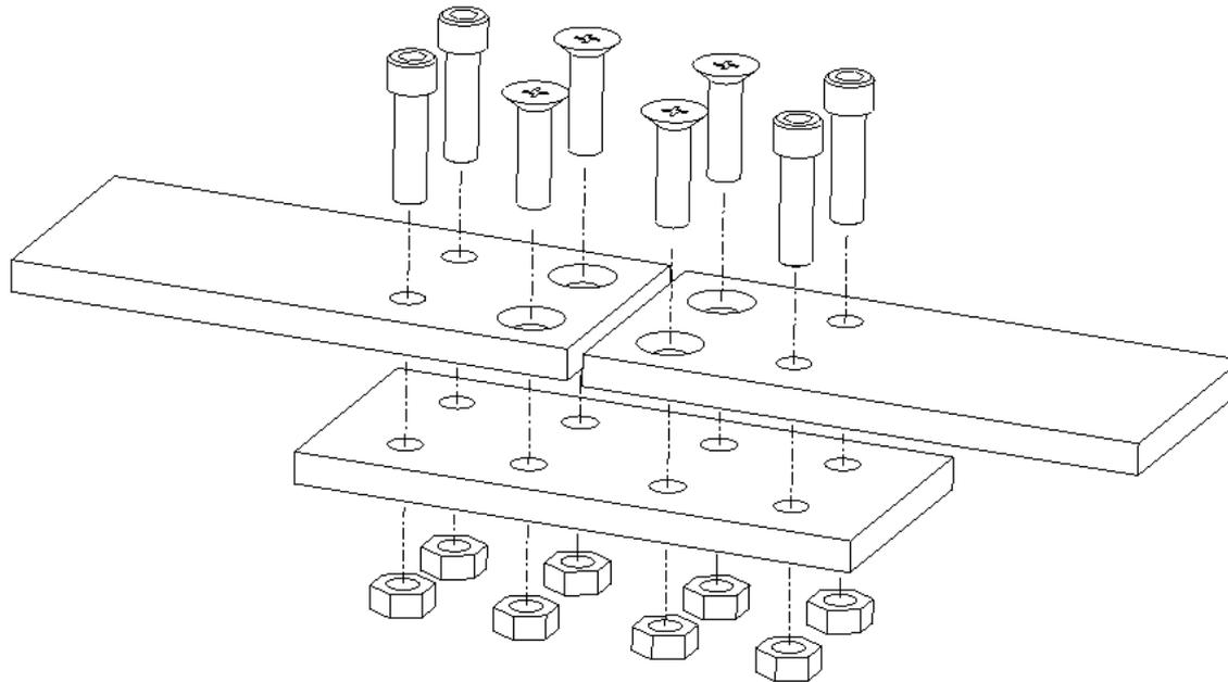
8 stainless steel fasteners (4 with countersunk heads, and 4 with socket heads)
