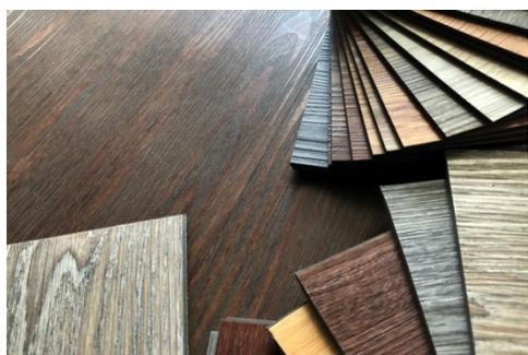
Luxury vinyl tile flooring (LVT) is made as either glue-down or floating tiles and/or planks. Four distinct layers are fused: a resilient vinyl backing, a vinyl photographic film layer, a performance wear layer, and a urethane or aluminum oxide top layer for wear/scratch resistance.
